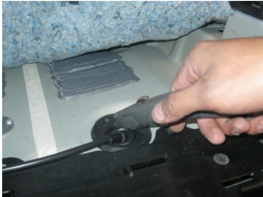
Figure 22. Example grommet pass through location.
