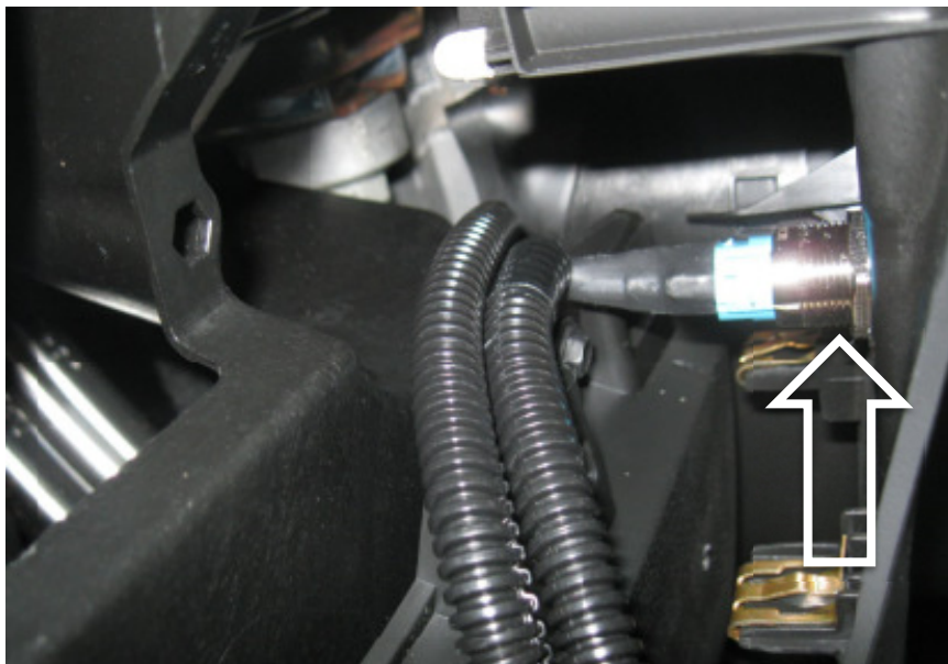
Figure 21. The jam nut on the back of the manual pump operation button.
