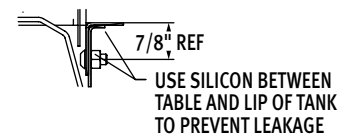
Sectional View Showing Table Connections
