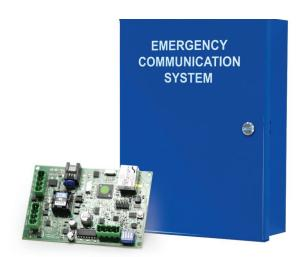
The Dialer Board allows emergency calls to be sent from a Shield30 Master Command Panel to a standard phone line.
