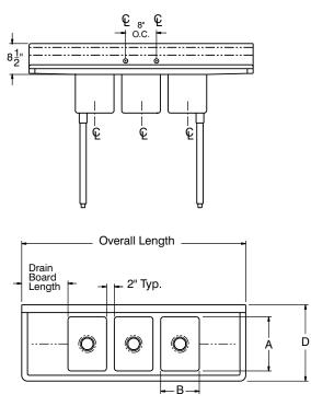
3 Compartment Sink with 2 drainboards Shown
