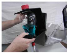
Secure the funnel stopper by positioning the retainer plate above the stopper and tightening the knurled nut. The funnel is now secured and can be inverted for shaking by loosening the knob. Make sure the holder is tightened securely before operating the shaker.
