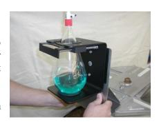
Install the front two holders onto the shaker platform. The "lazy Susan" platform rotates to make loading and unloading of holders and glassware easy. Pull the knurled knob near the center of the platform in an upward motion with one hand and rotate the platform with the other hand. Release the knurled knob when rotation of the platform has begun. When the platform has rotated 180 degrees, the plunger of the knob will lock the platform into place.
