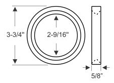
This gasket is a direct replacement for the 4" Cherne "Original", End of Pipe Gripper Mechanical Plug seal that serves as the blackwater tank stopper on Prevost Class A Motorcoaches. Saves you money by reusing the existing plastic and metal parts. Other places you may find this seal is with drain, water, and vent applications.
