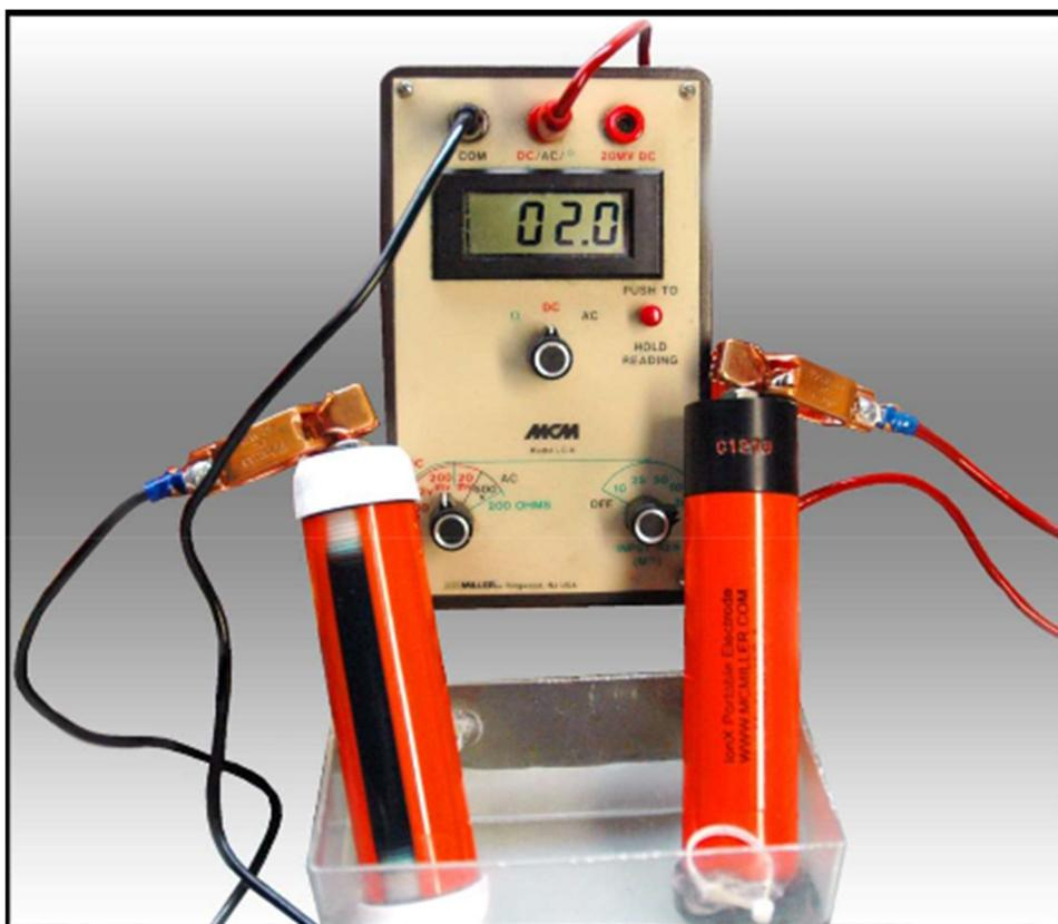
Since the IonX electrode potential was quoted as 318mV versus SHE on its Calibration Certificate, and, since the voltmeter reading (potential difference reading) was indicated as 2mV (see the LCD in the above photograph), the electrode potential of the RE-5C electrode, in this example, would be inferred to be 316mV versus SHE (318mV minus 2mV).
