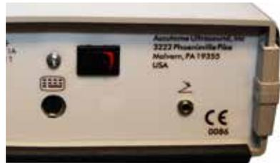
Figure 3.2 - Footswitch and Keyboard Connector
