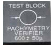
Figure 3.7 - AccuPach VI Test Block (top of instrument)
