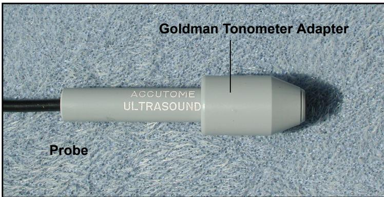
**Figure 12** *Probe with Goldman Tonometer Adapter*
