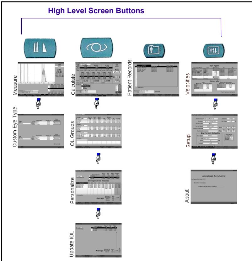
Figure 32 Accutome A-Scan Plus Screen Hierarchy
