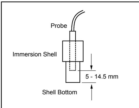
Figure 11 Probe Setup with Immersion Shell
