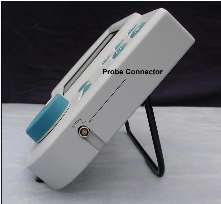
**Figure 7** *Probe Connector (Right Side of Instrument)*
