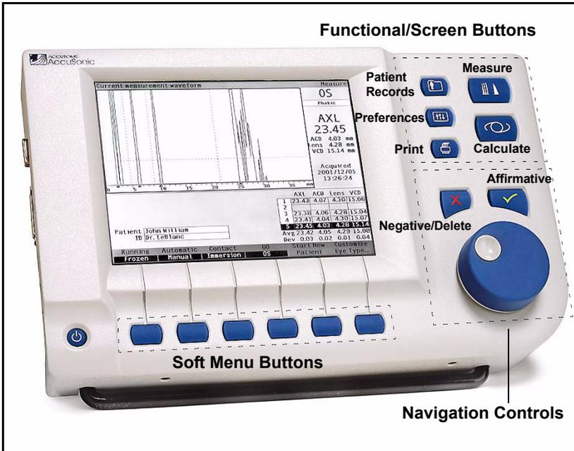
Figure 31 Accutome A-Scan Plus Buttons
