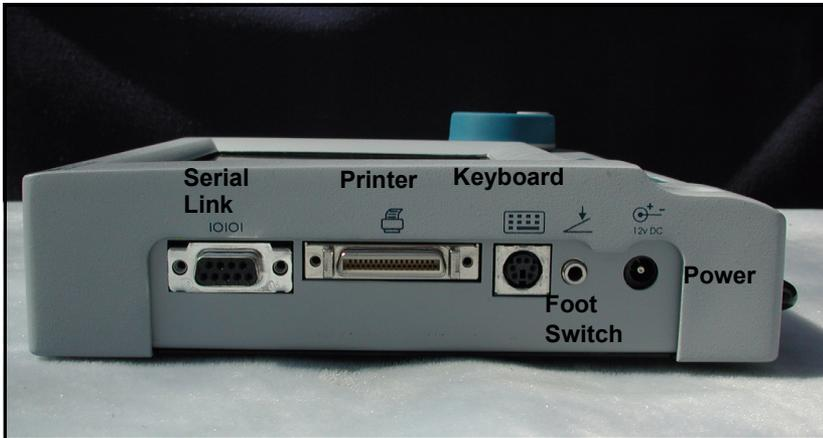
**Figure 6** Component Connectors (Left Side of Instrument)
