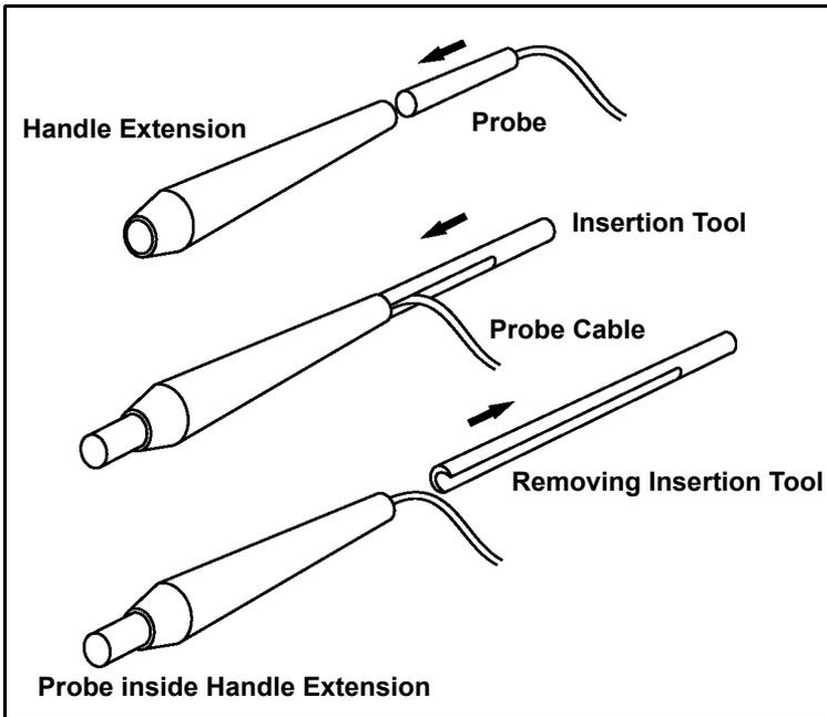
Figure 13 Inserting the Probe into the Handle Extension
