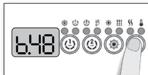
Use the Up/Down key to select the breaker value. The value can be modified from 10 to 48 A.
