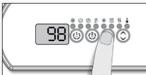
Press and hold the Program key for 20 seconds until you access the breaker setting menu.
