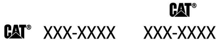
Figure 13 – Acceptable Cat Design Mark Locations Relative to Cat Part Number, Similar for Yellowmark Symbols used with Yellowmark Part Numbers
