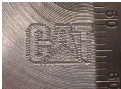
Figure 10 – Design Mark Reproduced Via Pin Stamping
