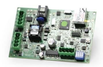
The Dialer Board allows emergency calls to be sent from a Shield30 Master Command Panel to a standard phone line.
