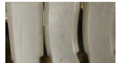
CastGuard™ after 2000 salt spray hours*
