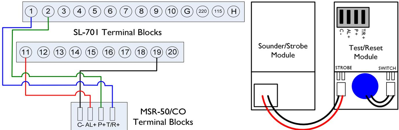
The SL-701 provides a 2 amp form "A" alarm contact and a 10 amp form "C" trouble contact for fire alarm control unit monitoring. The SL-701 will give a trouble report if the unit loses power, if the cover is removed, a sensor "end of life", or improper installation of the sensor.
