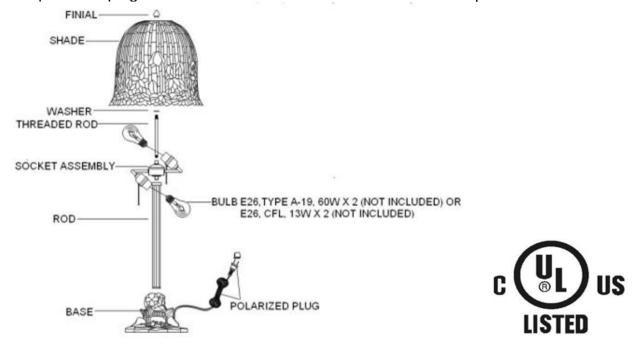
Note: The diagram illustrates the installation of your new luminaire. This is a representative drawing and is not intended to match the style of your luminaire.
