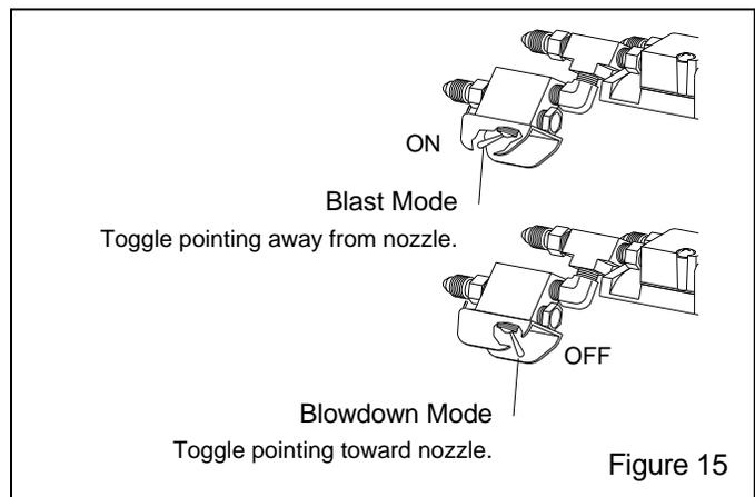
**3.6.2.2 Blowdown Mode:** Moving the ACS toggle toward the nozzle to the OFF position cuts off the control air to the abrasive metering valve, closes the valve, and stops the abrasive flow. This action allows air alone to exit the nozzle, useful for clearing the blast hose before shutting down, and blowing abrasive and water off the blasted surface.
