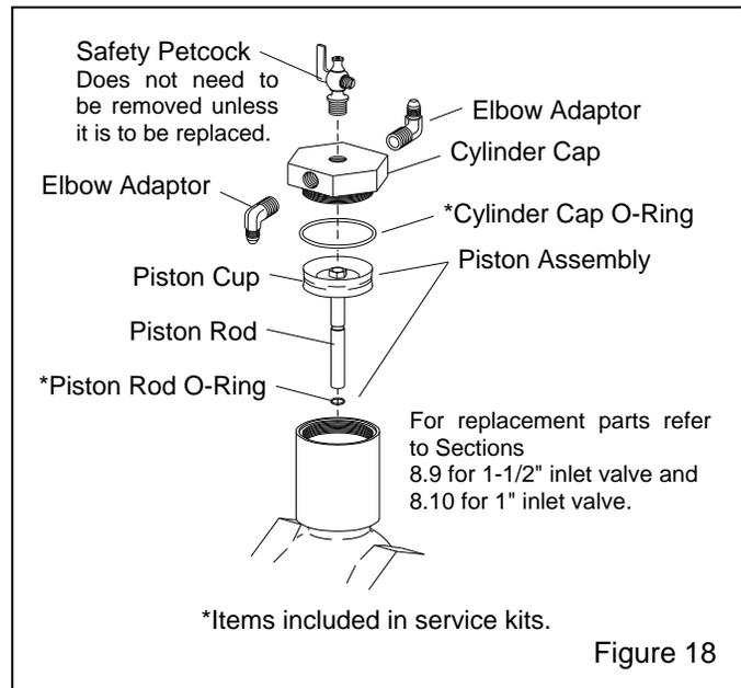
**6.3.2.6** Lubricate the cylinder wall and piston cup with lightweight machine oil or tool oil.
