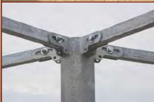
A 8½" diameter steel tower, made from ½" steel pipe. Brackets are fully welded into place and slotted for easy assembly.
