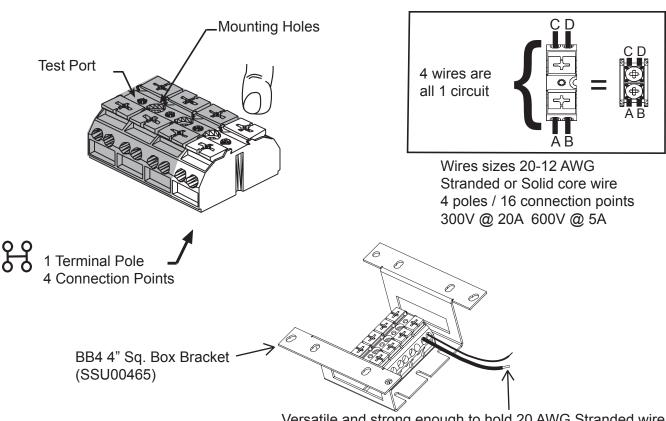
Versatile and strong enough to hold 20 AWG Stranded wire under 1 point and 12 AWG Solid under the second point.
