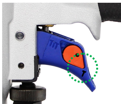
Selector Arrow set to Full Sequential Actuation Mode
