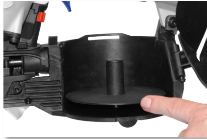
Set the plate level in the magazine depending on the nails' length.
