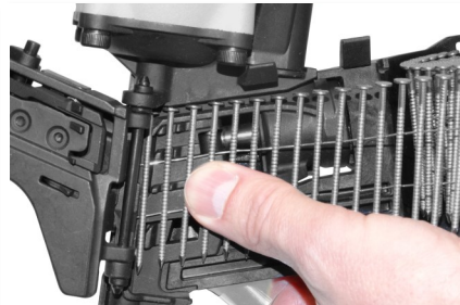
Load the coil nails in the magazine. Line up the end with the nose, and keep the nails' heads in the slot.
