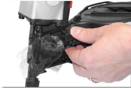
Push the latch until unlocked.
