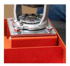
2. Using a socket wrench, tighten the bolts. Repeat this step on all 4 wheels at every corner.
