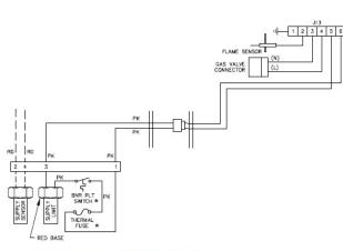
\* may require a jumper wire if unit is not equipped with fuses
