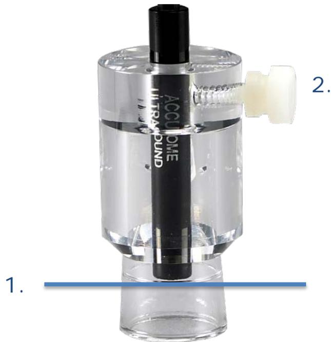
1. Insert probe through the hole on the top of the immersion shell. Do not push the probe past the scored line.
