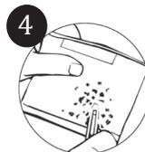
4 Extract the sample by thoroughly macerating it with an Agdia tissue homogenizer or a blunt object such as a pen or marker. An adequately extracted sample will result in a homogenous green or light brown colored solution. Allow the resulting solution to settle for 3 minutes before inserting the ImmunoStrip.
