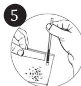
5 Remove an ImmunoStrip then reclose the container. When handling the strips, always grasp the top of the strip marked with the test name. Do not remove the protective covering.
