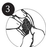
3 Insert the sample between the mesh linings near the bottom of the sample extraction bag.
