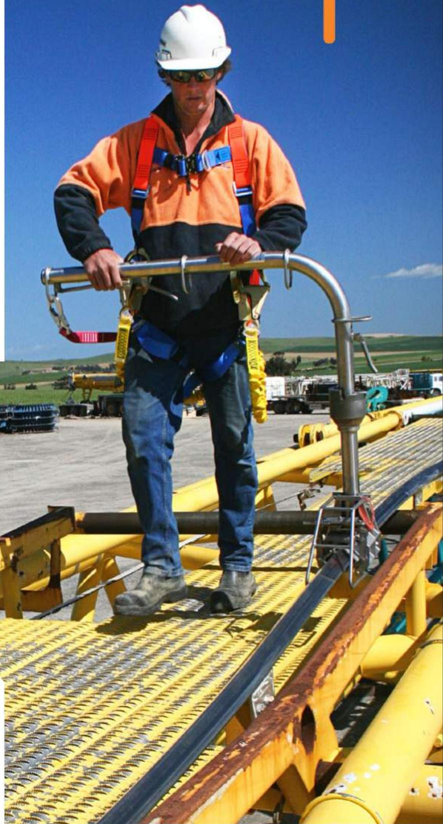
The TRAM system is designed for use on all crane types – telescopic or lattice boom, gantry or tower – and most other construction machinery.
