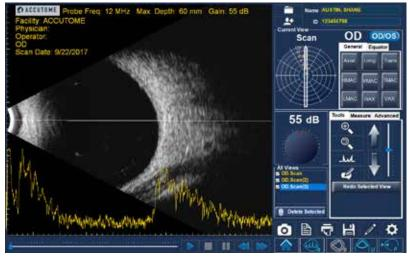
Figure 10.10 - B-Scan with A-Vector Overlay
