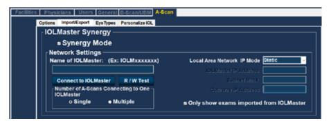
Figure 6.3 - A-Scan Synergy Mode Setup Screen
