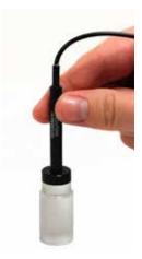
Figure 9.6 - Using the A-Scan Test Block
