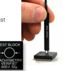
Figure 11.2 - Using the Pachymetry Test Block
