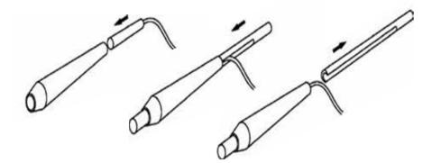
Figure 9.4 - Inserting Probe into Probe Handle Extension
