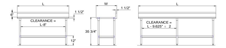
All units ship unassembled for reduced shipping cost. Units 7 ft. and larger are furnished with six legs. All dimensions are typical. Tolerance +/- .500". Finished size of undershelf. Shelf length = length minus 4.875" Shelf width = width minus 4.25"
