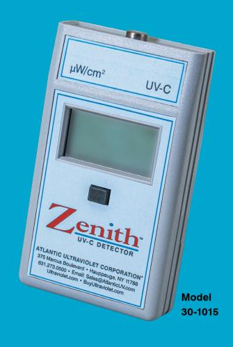
Using the **Zenith**<sup>™</sup> UV-C Detector, test along the fixture's seams, covers, duct work, light traps, or any area which appears that light can be escaping. Ideally, the **Zenith**<sup>™</sup> UV-C Detector should display "0" in all cases and at all distances.
