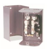
The MR-199 Series Heavy Duty Power Relays provide DPDT 30 Amp contacts which are operated from either a 120VAC or 24VDC control input. These relays are designed for control applications where 30-AMP DPDT contacts are required. Two models are available; a 120VAC coil and a 24VDC coil each of which may be mounted in a rugged steel enclosure.
