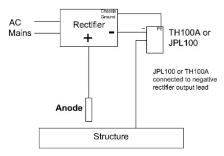
• Switching on the positive side of rectifier
