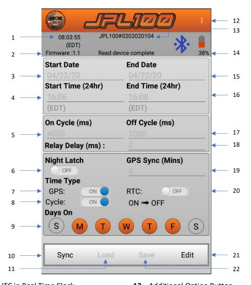
**UTC in Real Time Clock** 12 Additional Option Button 1 2 Firmware Version **13** Serial Number 3 Start Date **14** Battery Percentage 4 Start Time 15 End Date 5 **16** End Time On Cycle Night Latch **17** Off Cycle 6 **GPS Mode Selector** 7 **18** Relay Delay 19 GPS Sync Period 8 **Relay Position Switch** 9 Weekday Selector 20 RTC Mode Selector
