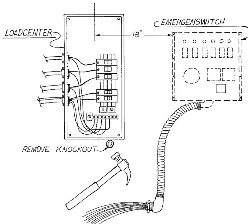
3. Identify an appropriate knockout to remove: 3/4" for the 6-circuit models and 1" for the 10-circuit models.
