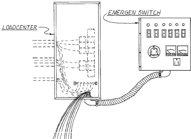
4. Insert the wires from the flex conduit up through the knock-out; take care to not nick or gouge the wires on the metal edge. Tighten the locknut securely onto the load center. The wires can hang freely.
