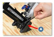
Loosen the four screws (A) and push the two stabilizing feet up to the highest position, then tighten these screws slightly.
