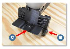
Loosen triangle base screw (B).
