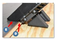
Push two stabilizing feet down until the are in full contact (E) with the hardwood flooring surface.
