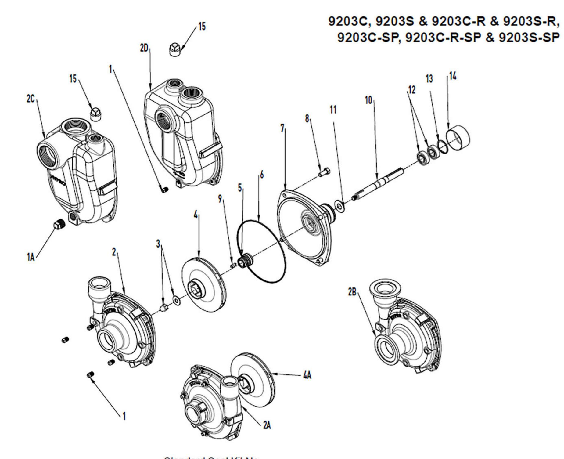
Silicon Carbide Seal Kit No. H3430-0589 consists of: (1) Ref. 5 Mechanical Seal (1) Ref. 6 O-Ring Standard Seal Kit No. H3430-0332 consists of: (1) Gasket (not shown) (1) Ref. 5 Mech. Seal (Viton) (1) Ref. 6 O-Ring
