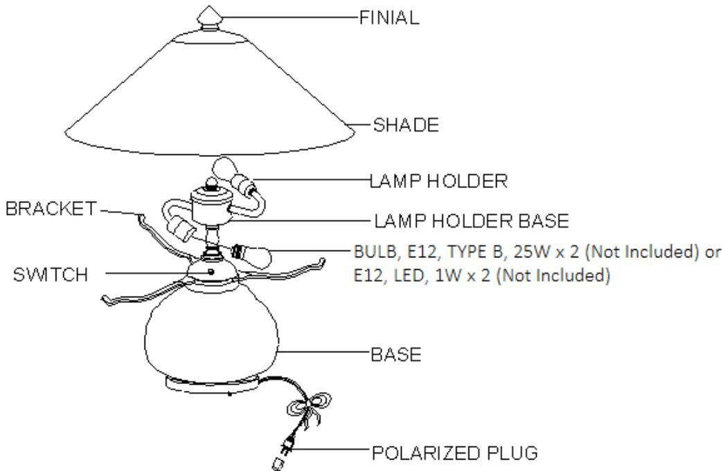
**Note:** The above diagram illustrates the installation of your new luminaire. This is a representative drawing and is not intended to match the style of your luminaire.
