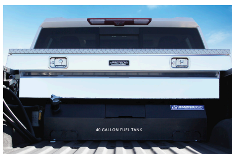
The compact design of our 40-gallon fuel tank fits under most over-the-bed-rail tool boxes, including those made by ProTech.
