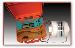
Measured Resistance =  $118 \Omega$ Resistivity Value =  $118 \Omega \times 16.25$  cm =  $1,917.5 \Omega$ .cm [Hence MCM Tap Water Conductivity =  $521 \mu$ S/cm]
