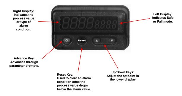
Figure 3. Digital Control Module Detail
