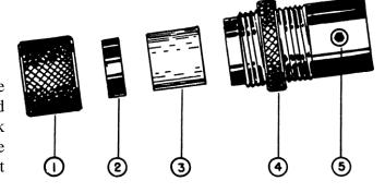
Unscrew the collar (1) from the chuck and remove the pressure ring (2). Place the flexible insert (3) into the chuck and replace the pressure ring with the counter bored end facing away from the flexible insert. Screw the collar back on the chuck but do not tighten.
