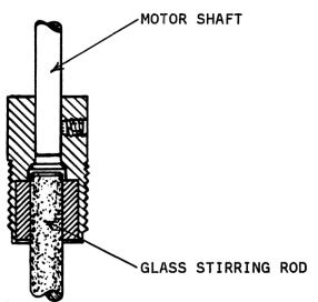
Loosen collar just enough to insert pestle to full depth, then withdraw approximately 2mm to allow for movement of rod due to misalignment. DO NOT ALLOW MOTOR SHAFT TO TOUCH GLASS PESTLE ROD. Make sure pestle is aligned with motor shaft then tighten collar as tight as possible by hand and lock in position with locking ring (4).
