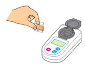
Measure the absorbance of each test tube at 470 nm. Calculate concentration of histamine in samples using their absorbance and an equation.
