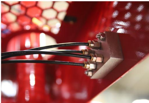
The centrally located grease port allows for ease of maintenance.
