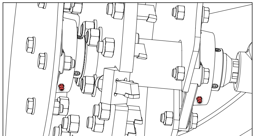
Flywheel Shaft Bearings (Underside of Flywheel Housing)
