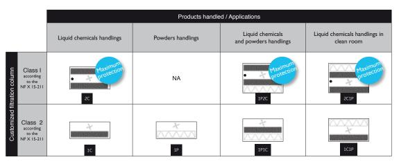
Carbon filtration for gases and vapours
