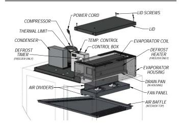
FIGURE 9B: Roll-In Refrigeration System
