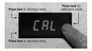
Once you see this, press on the front lower left to decrease temperature displayed, or on the upper left section to increase temperature displayed. After adjusting the offset, press the right center of the front display again to exit calibration mode. Wait 10 to 15 seconds for the cabinet temperature to appear and recheck the display calibration.
