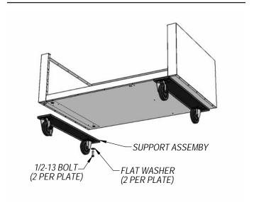
Using the small holes in the plate as a template, drill 1/8 pilot holes in the bottom of the cabinet. (Note: drill only until you penetrate the metal bottom of the cabinet. Do not continue to drill into the insulation, or you may damage the cabinet.) Secure the caster support plate assembly to the cabinet with a sheet metal screw in each of the drilled holes. Tighten the 1/2" bolts. Repeat these steps to attach the other plate assembly to the opposite end of the cabinet.
