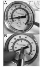
(+/- 1°C). If it does not, use a small straight-blade screwdriver to carefully pry the clear lens cover from the thermometer body as shown (see Photo A).
