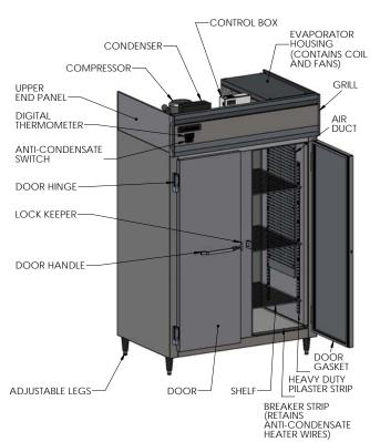
FIGURE 2B: Roll-In or Roll-Thru Refrigerator or Freezer
