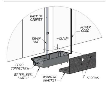
**IMPORTANT:** It is extremely important that the water level switch operates correctly, that the vaporizer is plugged into the receptacle labeled "VAPORIZER" and the compressor is securely plugged into the receptacle labeled "CONDENSING UNIT". Improper installation may cause your cabinet or vaporizer to operate "erratically." This can result in water overflowing the pan and onto the floor.
