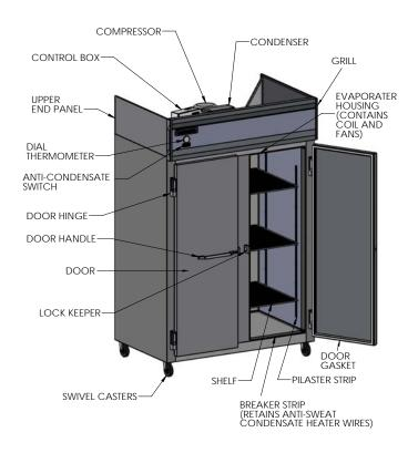
Standard Reach-In refrigerators and freezers have an internal evaporator coil located behind the fan panel on the inside ceiling of the refrigerated compartment (see Figure 2). Designer Line Reach-In, as well as all Pass-Thru, Roll-In and Roll-Thru refrigerators and freezers have an insulated housing located on top of the cabinet, that contains the evaporator coil, out of the refrigerated storage area (see Figure 2A & 2B).
