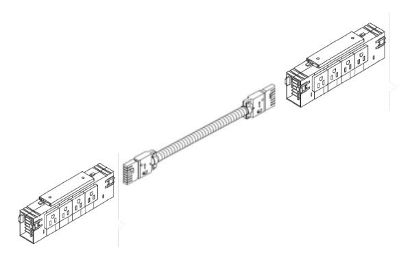
Open-wire starter harnesses come in 72" and 168" lengths and are hardwired to the electrical system of the building. Electrical harnesses are available in singular lengths ranging from 19" to 145" at 3" increments, or as a combination of two harnesses up to 181" in length.
