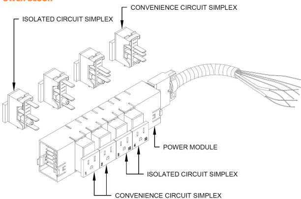
Isolated receptacles are made evident by their orange color. Electrical harnesses have a metal flex casing to prevent interference with voice/data cabling, and shield all electrical wires. Electrical harnesses easily snap together to make a connection. Power modules can be installed or relocated without dismantling the panel.
