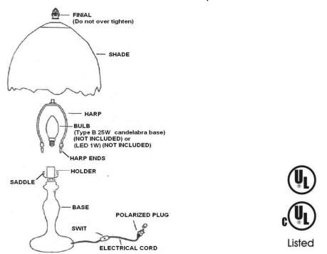
Note: The diagram illustrates the installation of your new luminaire. This is a representative drawing and is not intended to match the style of your luminaire.
