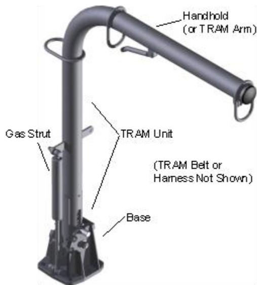
Figure 1: TR-02-01 Fixed Base TRAM w/ Standard Arm Shown
