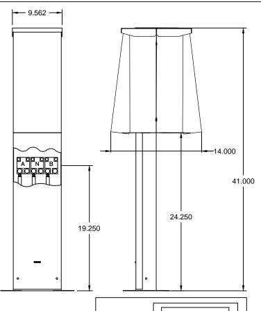
ETL-Certified, NEMA type 3R rainproof enclosure. One piece construction from G90 galvanized steel. All surfaces have electrostatic gray powder coated finish. 120/240 volt single phase, 120 Amp.
