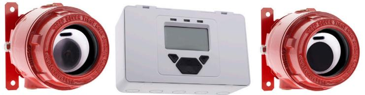
The Fireray® 3000 Exd is ideally suited for the protection of large areas, with potentially explosive atmospheres, against smoking fires. Fireray® 3000 Exd comprises an infrared transmitter and a receiver, both of which are ATEX-certified for use in Group 2 hazardous areas. There is a separate, safe area, wall-mounted remote/low level control unit to allow adjustment and testing from a convenient non-hazardous location.
