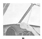
Lubricate the ¼" glass groove with glass lubricant or very soapy water to allow the glass to center itself while installing. Place new rubber on glass making sure that it is placed correctly and fits well. Any problems with fit will show up at this point. Rubber should fit glass without being too loose or too tight. Improper size will pucker or fold in corners. Place chrome strips in top and bottom slots of rubber first. Next, position sides and lock-
