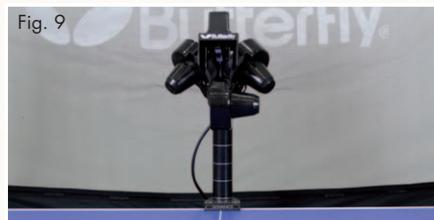
will automatically switch to the basic setting. The robot is now ready to deliver the balls to a specific point on the table. The landing spot can be continuously set using the rotary switch for left/right placement.
