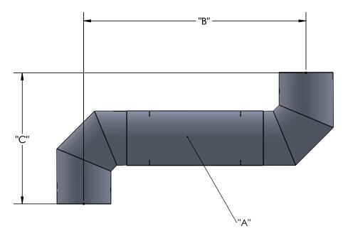
"A" REPRESENTS THE PIPE LENGTH BETWEEN THE TWO 45 ELBOWS FOR THE OFF-SET DIMENSIONS IN THE CHART
